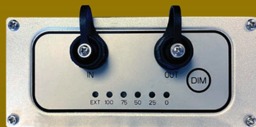
Onboard Dimmer & External Dimming connections
