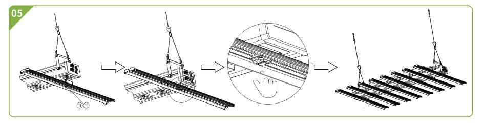
•Attach the light module to the chassis, press the button to lock.(Press again to remove the light module from the chassis.) The UV light module should be installed on the third and the sixth purple base .
