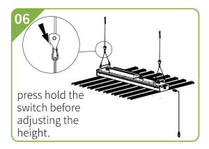
•Adjust the height by pull the cable.
