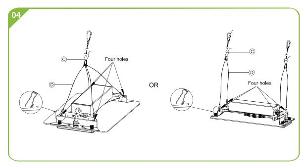
4. Hook the hanging cables  $\bigcirc$  to the fixture and the adjustable hanging rope(s)  $\bigcirc$  to the cables  $\bigcirc$ .
