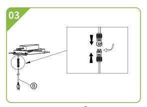
3. Connect the plugs **B**. Dial the switch to "♠" position to lock the cable.
