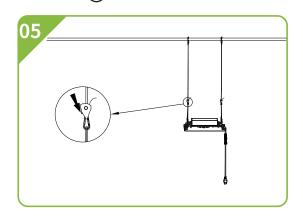
5. Hang the fixture to the desired installation location.
